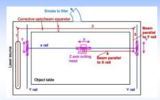
. Usually the head mirror is  $\lambda/4$  to transform polarized beam to circular polarized, => avoid asymmetric thickness of the track
